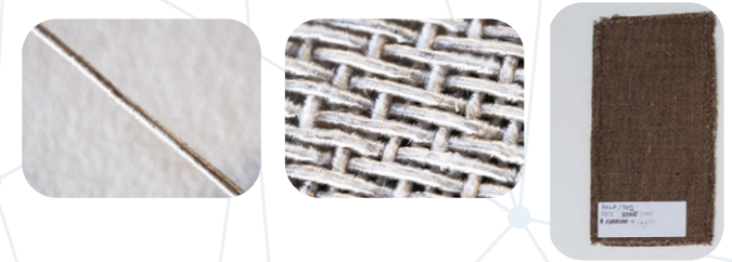
▲ Figure 14: Hybrid fabrics from comingled yarns and composite sample
