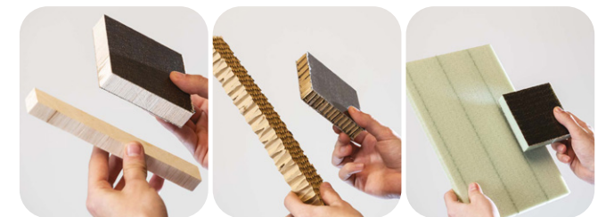
▲ Figure 19: Pictures of sandwich materials. Skins are made with woven hemp fabrics and GreenPox. The core materials are balsa wood, paper honeycomb and recycled PET foam (from left to right)
