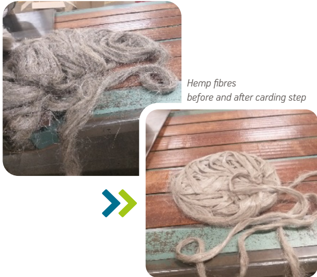
Figure 10: Production of hemp rovings
