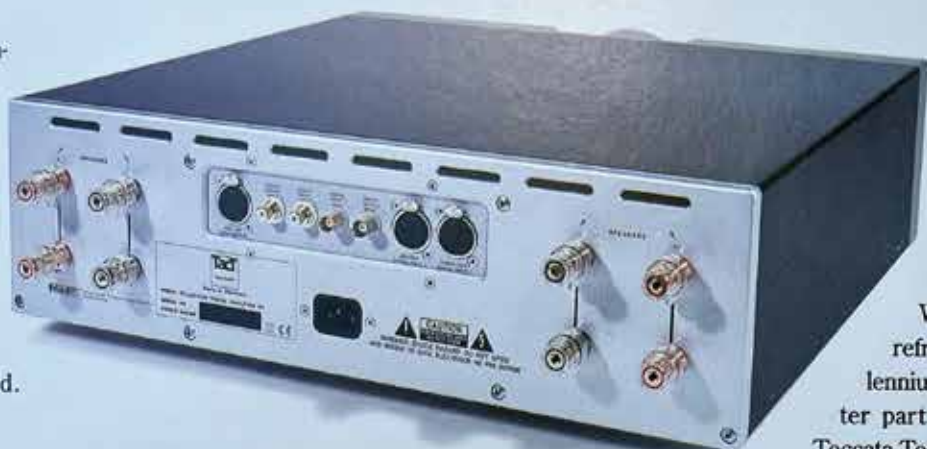
Behind the Millennium: A host of digital inputs and speaker binding posts.
