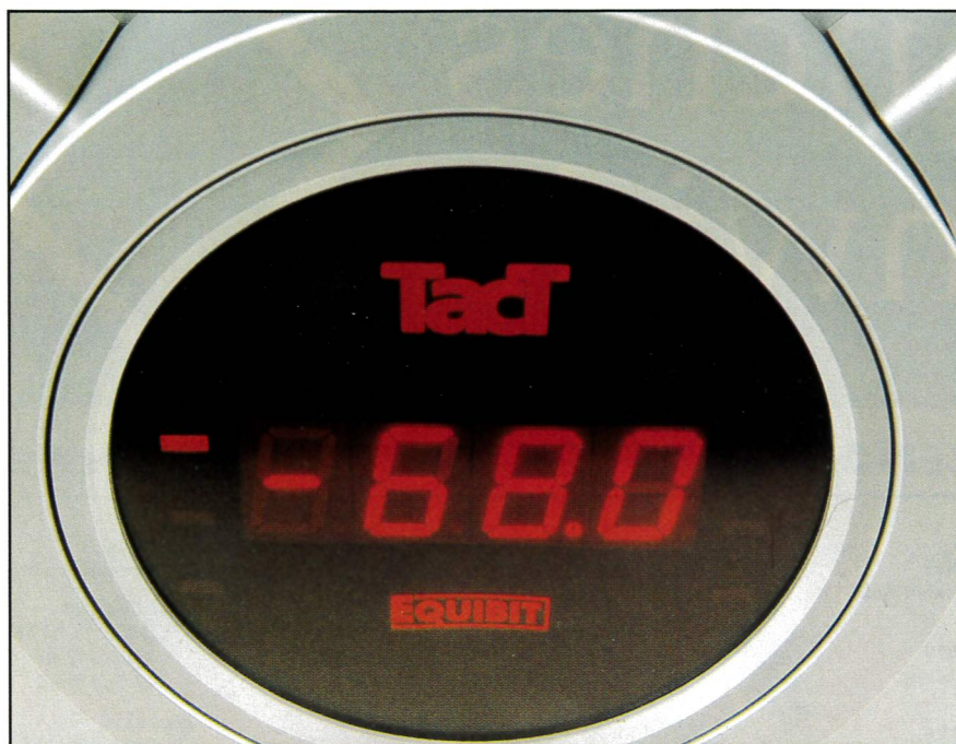
This is the Millennium's volume control wheel, which turns on military-specification bearings. The display indicates a nominal output level, ranging from -90 to +12.
